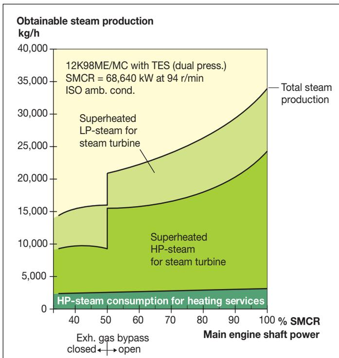
Fig. 12: Expected steam production of an exhaust gas boiler with a dual-pressure steam system valid for main engine 12K98ME/MC with TES and based on ISO ambient reference conditions
