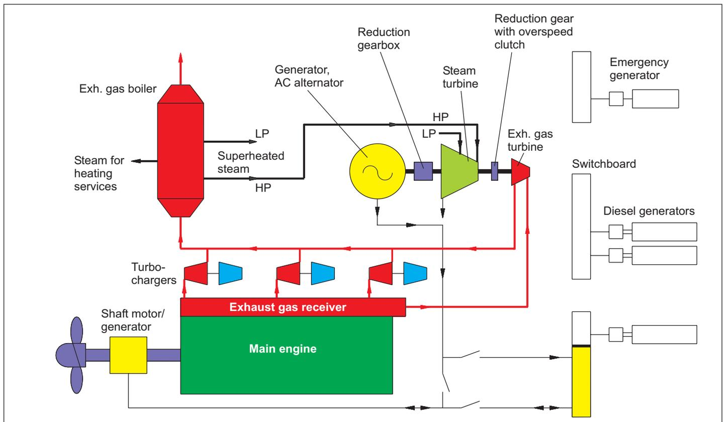
Fig. 2a: Power concept for the Thermo Efficiency System
