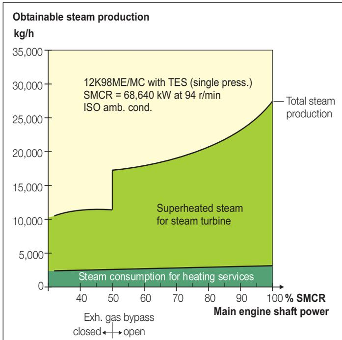
Fig. 10: Expected steam production of an exhaust gas boiler with single-pressure steam system valid for main engine 12K98ME/MC with TES and based on ISO ambient reference conditions
