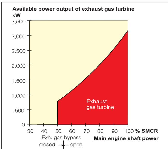
Fig. 8: Expected available power output of exhaust gas turbine for a 12K98ME/MC with SMCR = 68,640 kW x 94 r/min
