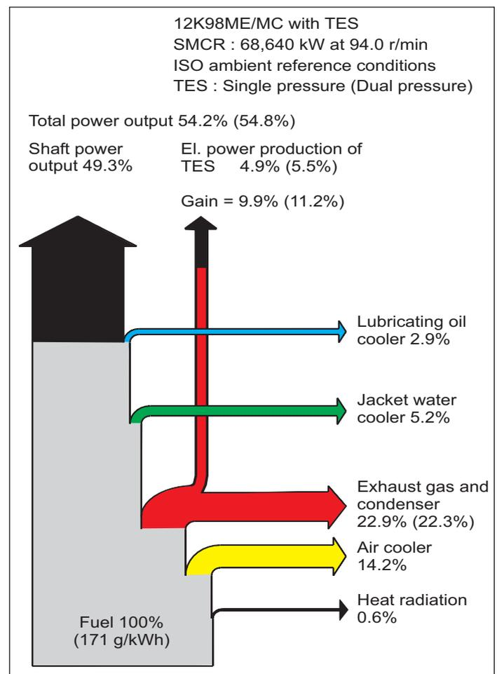
Fig. 1b: Heat balance diagram of the nominally rated 12K98ME/MC engine in Thermo Efficiency System (TES) version operating at ISO ambient reference conditions and at 100% SMCR
