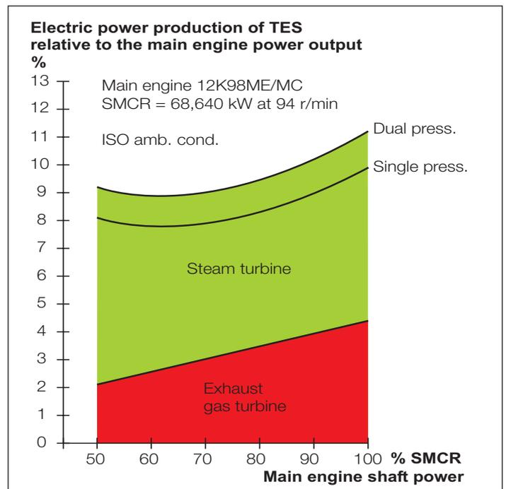
Fig. 9: Expected electric power production in % of the main engine shaft power output valid for a 12K98ME/MC with Thermo Efficiency System (TES) and based on ISO ambient reference conditions
