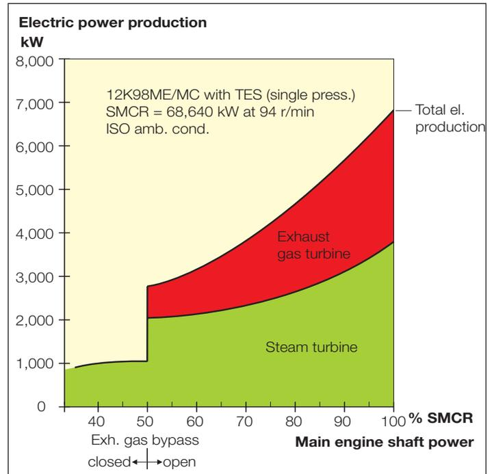
Fig. 11: Expected electric power production of the Thermo Efficiency System (TES) with a single-pressure steam system valid for main engine 12K98ME/MC and based on ISO ambient reference conditions
