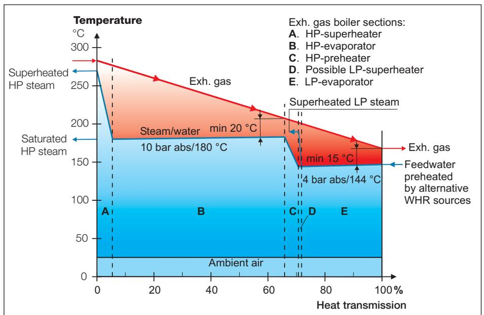
Fig. 7: Temperature/heat transmission diagram of an exhaust gas boiler with dual-pressure steam system valid for a main engine with TES and operating at 85% SMCR/ISO
