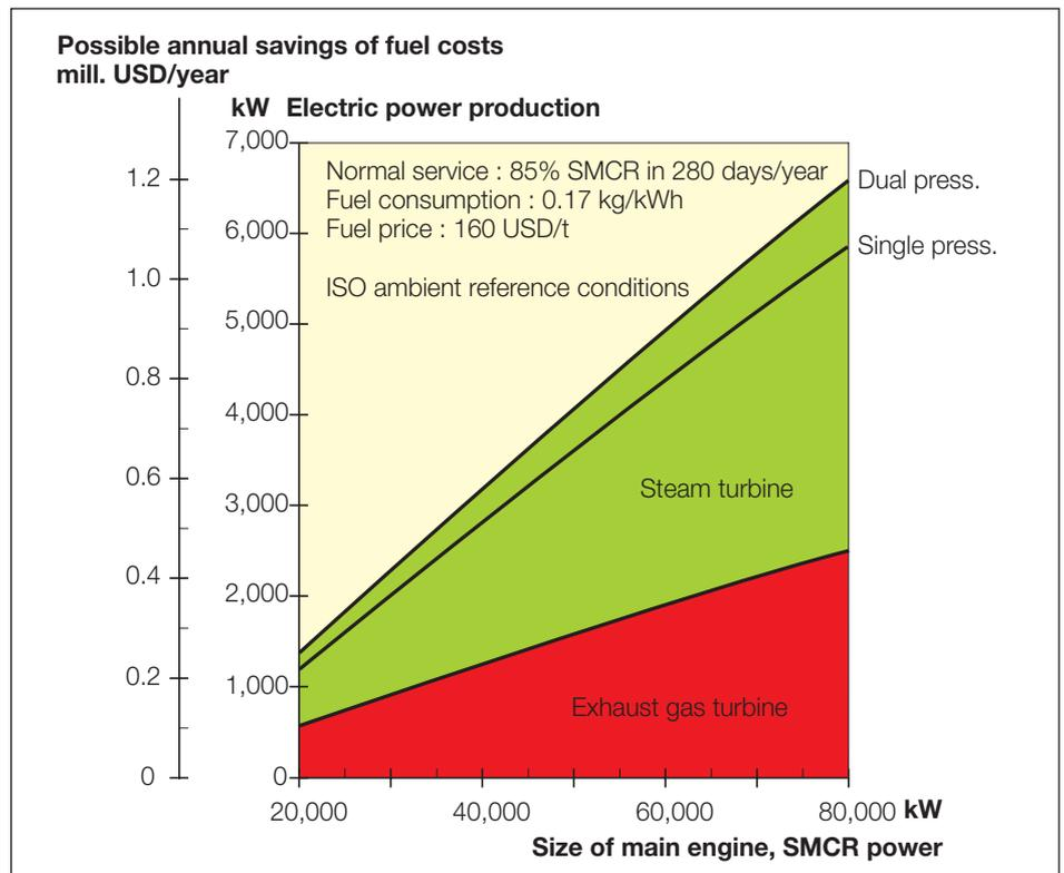
Fig. 16: Expected total electric power production and possible annual fuel cost savings of the Thermo Efficiency System (TES) based on ISO ambient reference conditions and 85% SMCR, shown as a function of the main engine size, SMCR power
