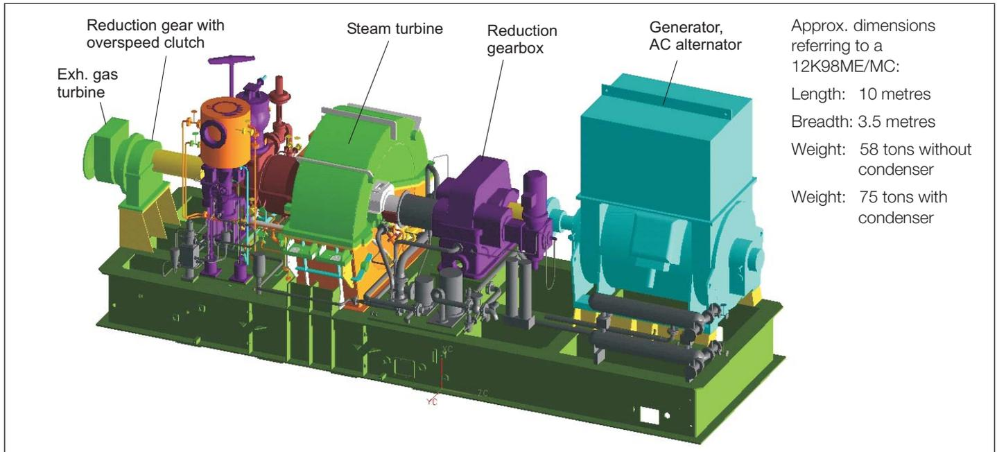
Fig. 2b: Arrangement of the complete turbine generating set as proposed by Peter Brotherhood Ltd
