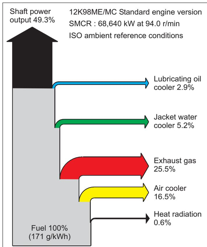
Fig. 1a: Heat balance diagram of the nominally rated 12K98ME/MC engine of the standard engine version operating at ISO ambient reference conditions and at 100% SMCR
