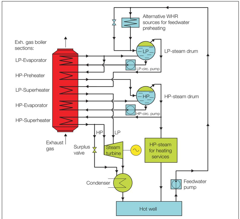
Fig. 6: Process diagram for the Thermo Efficiency System – dual-pressure exhaust gas boiler system with a dual-pressure steam turbine
