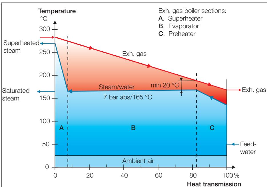
Fig. 5: Temperature/heat transmission diagram of an exhaust gas boiler with single-pressure steam system valid for a main engine with TES and operating at 85% SMCR/ISO
