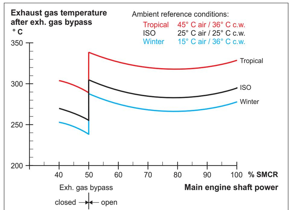
Fig. 3: Exhaust gas temperature after exhaust gas bypass for a main engine with TES
