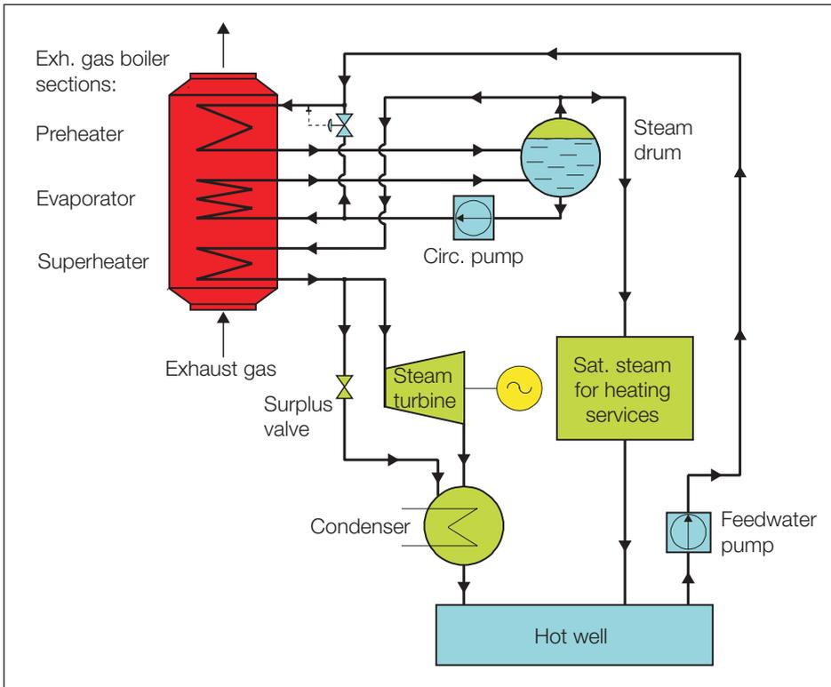
Fig. 4: Process diagram for the Thermo Efficiency System – single-pressure exhaust gas boiler system with a single-pressure steam turbine
