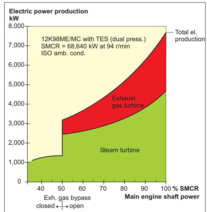
Fig. 13: Expected electric power production of the Thermo Efficiency System (TES) with a dual-pressure steam system valid for main engine 12K98ME/MC and based on ISO ambient reference conditions
