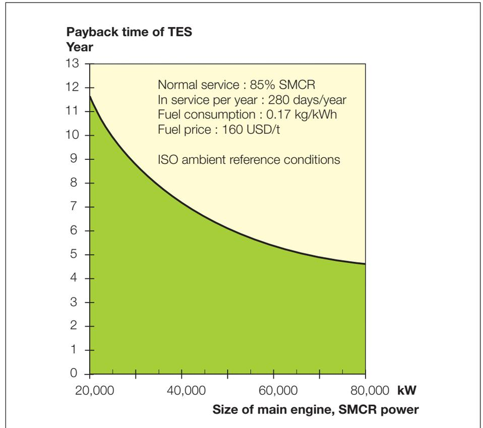
Fig. 17: Estimated payback time of the Thermo Efficiency System (TES) valid for both a single and a dual-pressure steam system
